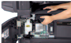
The TASKalfa 300i features high capacity toner rated for 20,000 pages (6% coverage)
